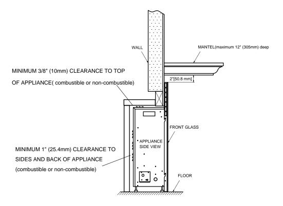
The fireplace insert may be placed within a framed enclosure that is level, dry, and capable of supporting the weight of the appliance and front glass. It may be placed directly on wood or a non-combustible surface (not on linoleum or carpet). The minimum clearance from the top of the appliance to a mantel (combustible or non-combustible) is 2" (50.8mm). The sides and back must maintain 1" (25.4mm) clearance to any material. The top must maintain a 3/8" (10mm) clearance to any material.
