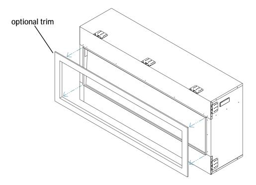
2. Remove the framing plates from the unit
