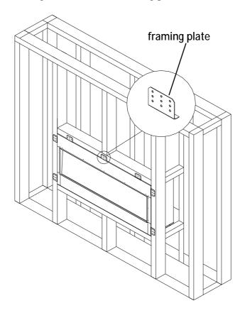
7. After checking that the fireplace operates properly, cover the glass panel with protective plastic bag and install polywood.
